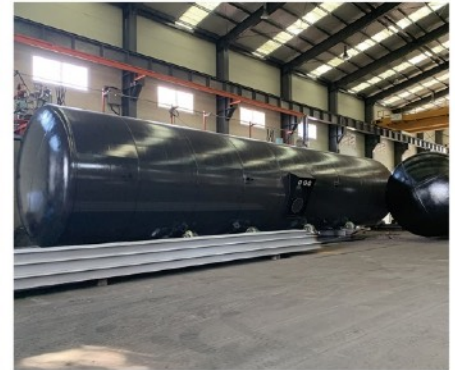
Underground Storage Steel Tank
